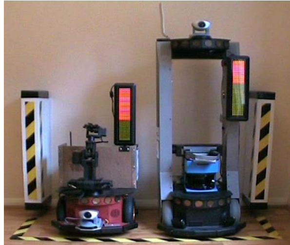
Figure 4.2 The LED displays indicate to the user that the companion is migrating between different embodiments (Pioneer and PeopleBot)
